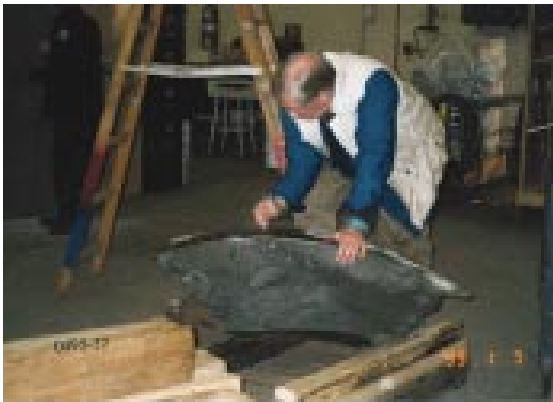
Staehle examines fragment from exploded pressure vessel.
